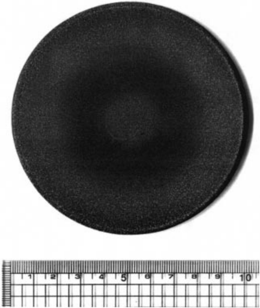
Fig. 5. Photograph of a 6% CH 4 diamond wafer.
